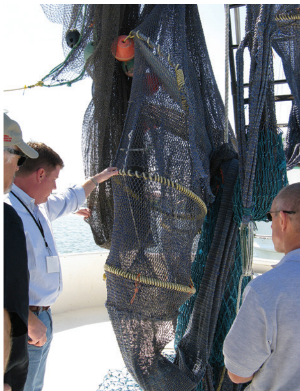
The top-performing Jones-Davis bycatch reduction device was developed by shrimp fishermen in Freeport, TX.
