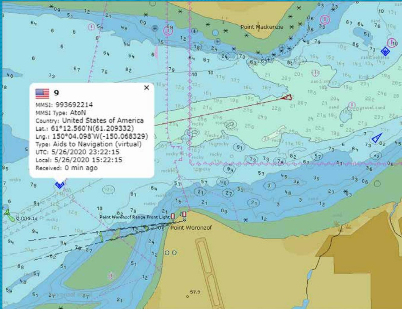
*Location of virtual buoy transmitted via AIS.*
