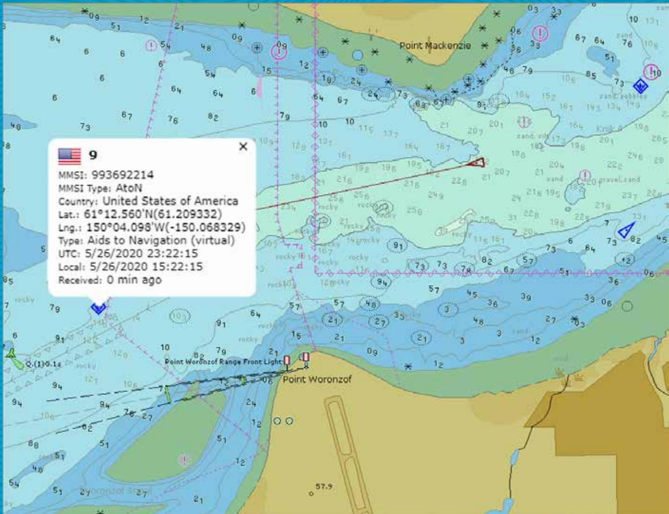
Location of virtual buoy transmitted via AIS.
